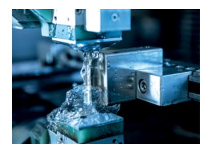
Wire eroding machines from Agie/GF and Fanuc traverse path up to 500 mm x 350 mm x 400 mm
